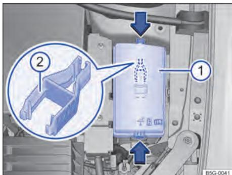
Fig. 169 No compartimento do motor: cobertura
